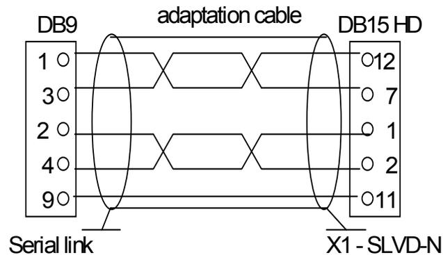
(\*) **Note:** the adaptation cable (DB9 – DB15HD) isn't included in the serial kit; the order code is: **SERIALTOSLVDN**.
