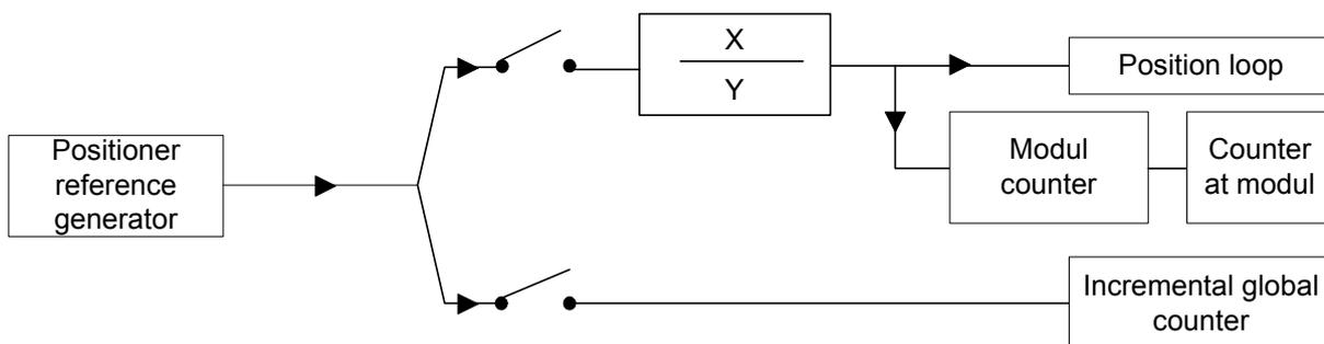
When the position reference of at least one generator is enabled in the position loop, the reference loading into a global counter defined by module is automatically enabled.
