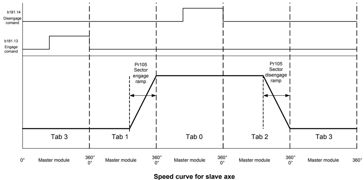
The above described tables are of course an example case to describe the engage and disengage functions of an axis by changing tables, and they are calculated in order to allow these functions for an axis that needs to be dynamically disengaged/engaged according to a gearing law ( $Pr102=5 \_ Y=5$ ).
