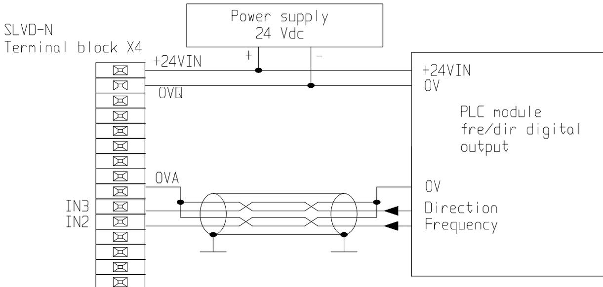
In the case it comes used a encoder external like reference, and this device is lacking in feeding, is possible to use IN2, of the terminal block X4, for feeding the device. You see following outline (connecting an external local power source, maximum 24Vdc, to pin the 11 of X4, "IN2", the tension is brought, inner, to pin the 11 of X2, "IN2").
