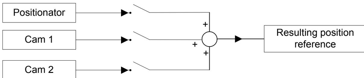
This diagram allows to identify a general flow in operating mode 11. If you carefully analyze this mode, you will see that the programmer can use several enabling commands (programmable bits) at different levels in order to address the flow of the generated position reference (or references), in several display modes. For instance, for each generator a position reference can be enabled in the position loop or into a general position counter.
