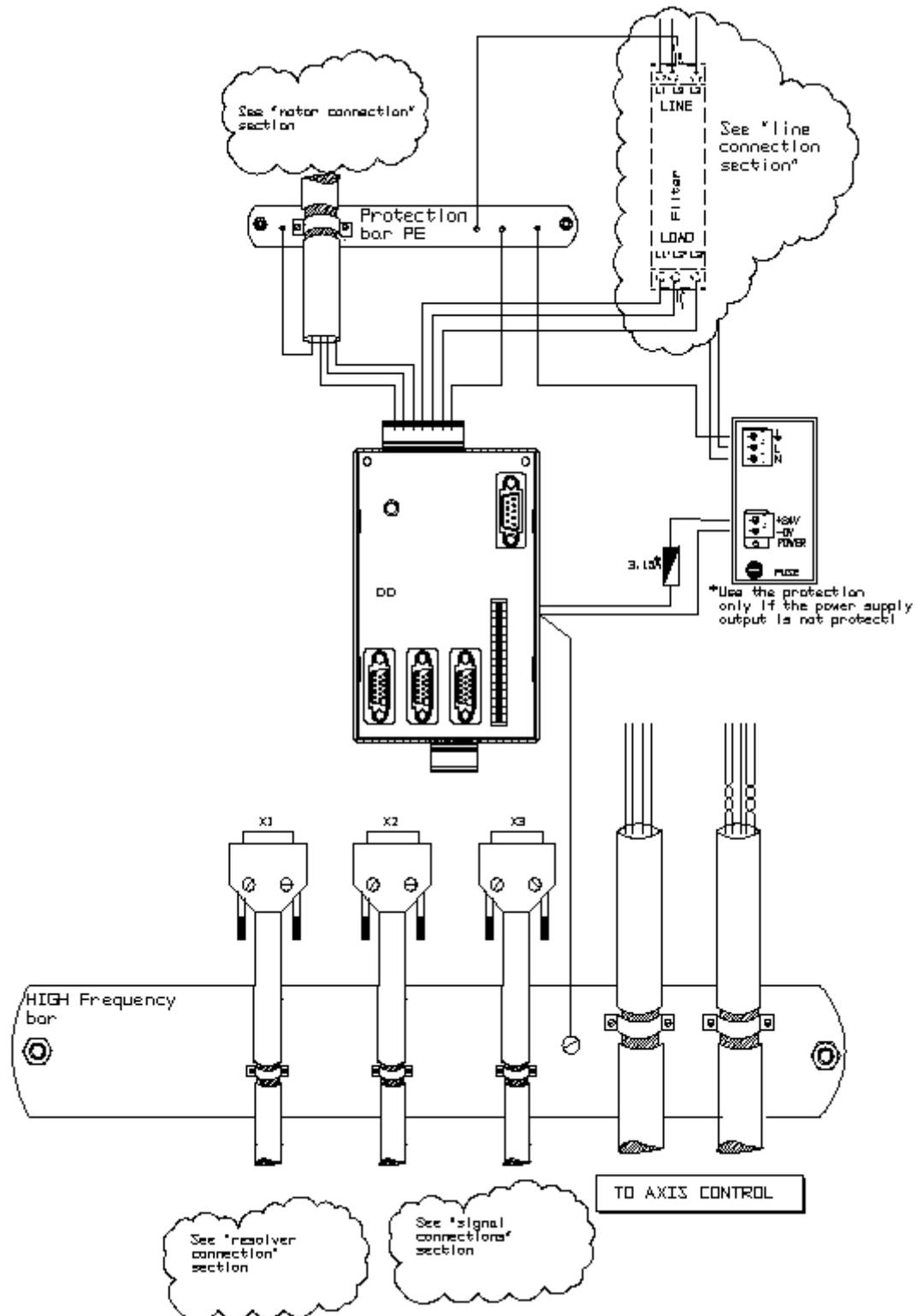
\* The PE bar (for power grounding) must be mounted directly in contact; insulated columns are not to be used.
