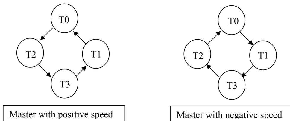
As shown in the figures, the table switching sequence is automatically inverted when the speed is negative.
