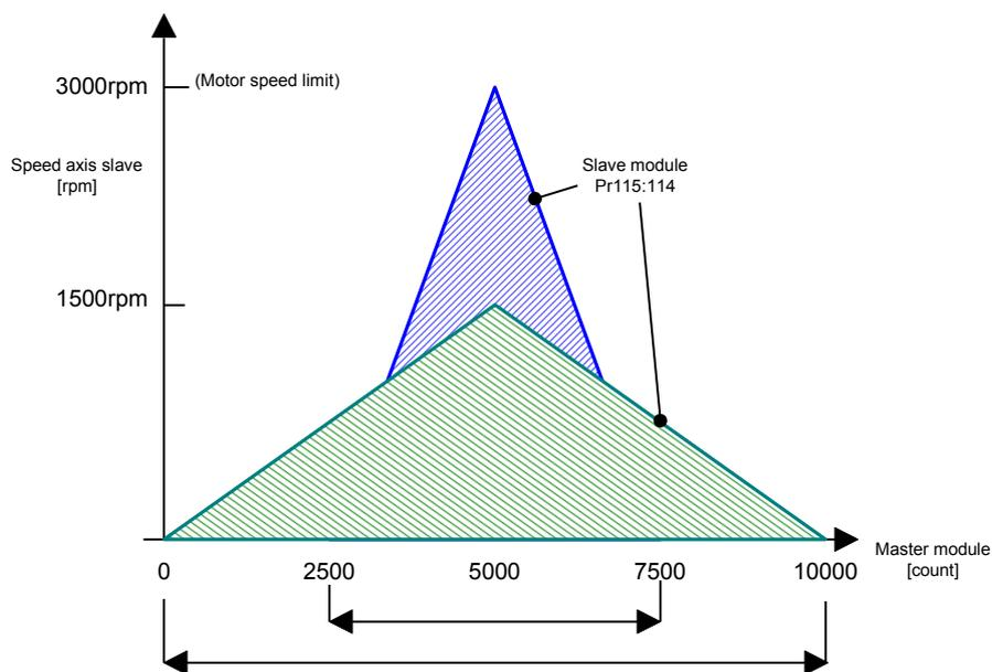
b150.12 and b150.13 command the engage and the disengage in correspondence of the master phases written in Pr127:126 and in Pr 129:128, they are always referred to master module of CAM1.
